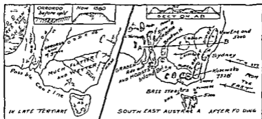
FIGURE 30—Drainage in south-east Australia showing changes in the rivers due to late Tertiary warping. Inset on the left are two vertical sections through Orroroo in the Flinders Horst.
